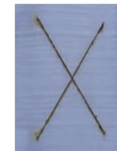
Primerless, one-coat Si-COAT 579 AC system applied directly to rusted steel.
