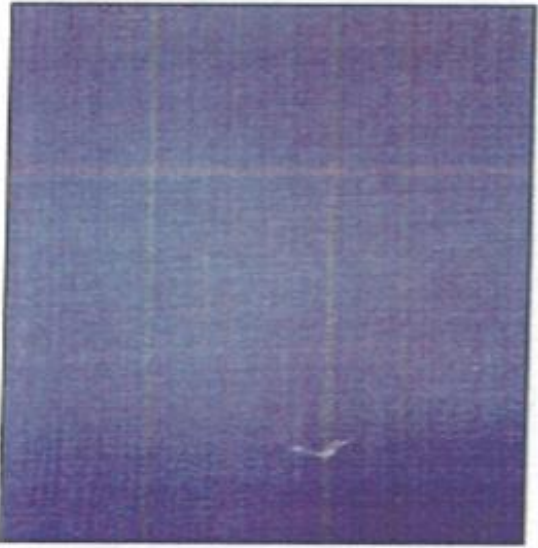
Figure 5: Cleaning with high pressure water at 200 bar begins to show slight damage to Si-COAT
